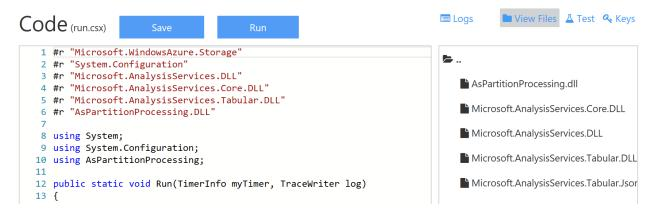
With the necessary class-library references in place, the function body can be written using SampleClient as a template. Again, PerformProcessing is the key method.
