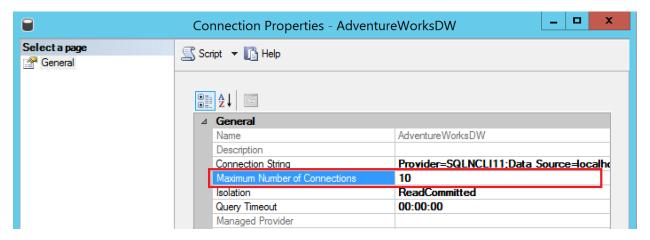
Analysis Services will determine the number of concurrent processing jobs based on the number of cores and available threads. These threads are shared across the server instance, and therefore one command may not receive all the available threads. The threads that do launch processing jobs may then be stalled to stay within the MaxConnections limit.
