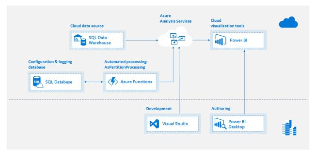
Azure SQL Database is used for the configuration and logging database.
